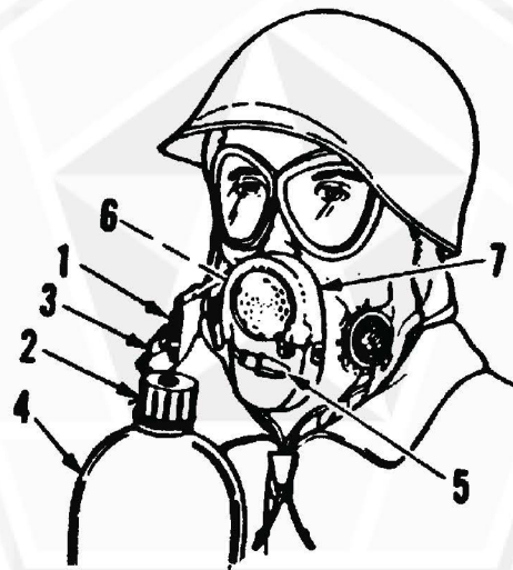
Fig 8-5. Disconnecting the drinking system.
