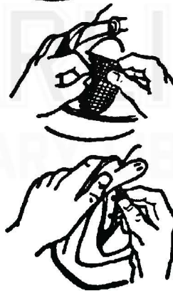
Fig 8-10. Installing filter elements.
